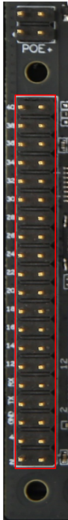
Figure 2. Astra Machina SL16x0 RDK board 40-pin connector pin definition
