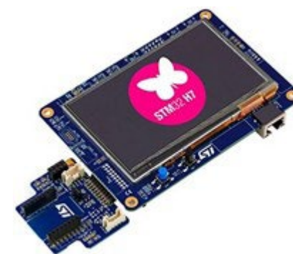
Figure 3: The STM32H745I-DISCO board integrates a wide range of on-board sensors and memory capabilities that allow developers to test out the dual core microcontrollers running at 480 MHz and 240 MHz. Image source: STMicroelectronics
