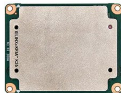
Figure 7: Production-optimized Kria 26 SOMs for industrial and commercial environments are designed to be plugged into a carrier card with solution-specific peripherals. Image: DigiKey
