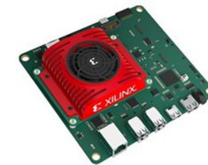
Figure 5: The Kria KV260 vision AI starter kit is a comprehensive development environment for machine vision applications. Image source: AMD Xilinx
