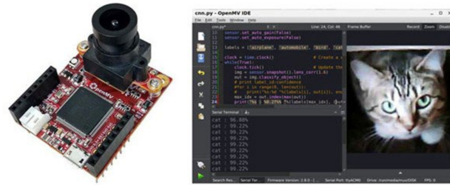
Figure 2: The OpenMV camera module can be used for image recognition, and development can be done with a simple IDE using Python. Image source: Benigo Embedded Group
