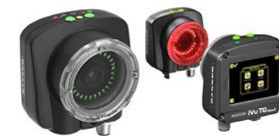
Figure 6: Image sensors from the iVu series can identify workpieces by type, size, location, orientation, and coloring. The machine-vision components can accept configuration and monitoring an integrated screen, remote HMI, or PC. Camera, controller, lens, and light are all pre-integrated. Image source: Banner Engineering Corp.
