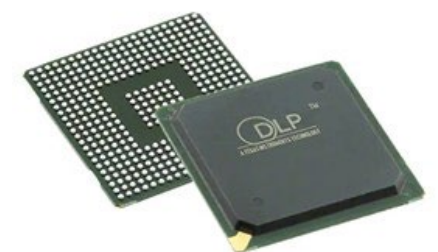
Figure 3: The DLPC350 integrated circuit (IC) controller provides input and output trigger signals for synchronizing displayed patterns with a camera. It works with digital micromirror devices (DMDs) designed to impart 3D machine vision to industrial, medical, and security equipment. In fact, applications include 3D scanning as well as metrology systems. Image source: Texas Instruments
