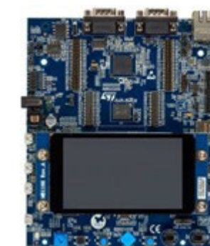
Figure 4: The STM32H757I-EVAL board provides developers with lots of expansion space, easy access to peripherals, and an LCD screen to get started with multicore applications. Image source: STMicroelectronics
